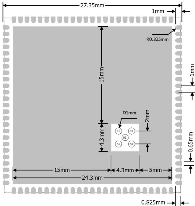
See figure above for the suggested module layout. The five 1mm pads in the square GND pad cutout can be omitted if no JTAG Boundary Scan test is used. The solder mask openings are shown below.
