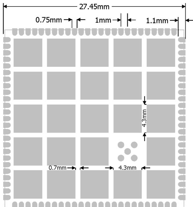
The ground pad solder mask on the bottom side of the QSCOM module is divided into sections for a better reliability of the solder joint and self-alignment of the component.
